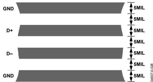
Figure 29. Arrangement of Signal Tracks
